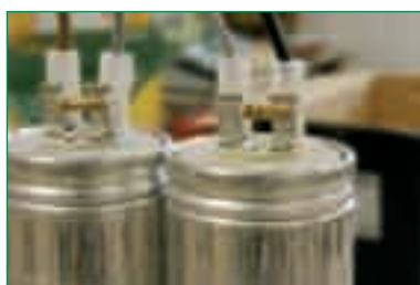
Detail of the automatic disconnection mechanisms and condenser discharge resistances.
