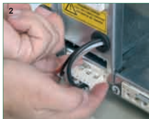
Remove quick connector
